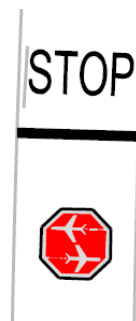
Marking on service road: full vehicle stop required
