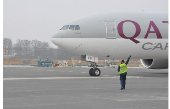
Marshaller providing sign that clearance is permitted
